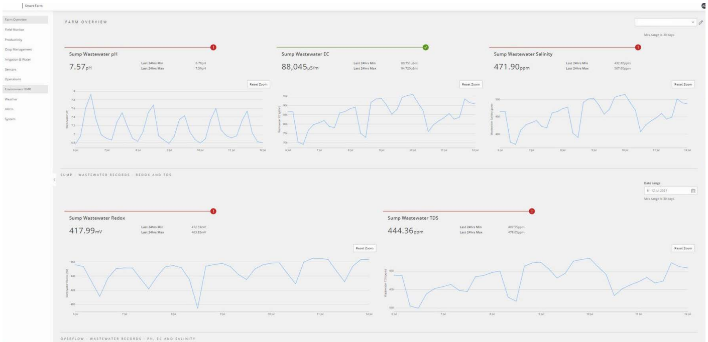
Example of the operations dashboard, showing wastewater parameters.
